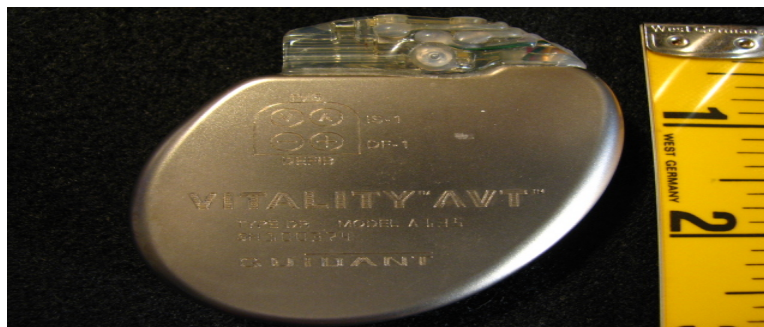
A real ICD/CRT-D generator (Guidant Vitality AVT) shown next to a ruler for scale — about the size of a wristwatch. The header at top is where the leads connect before the device is placed under the collarbone. Image: Steven Rodriguez, Wikimedia Commons 2007 (CC BY 2.0).
